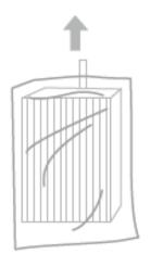
Remove the filter from the plastic protective packaging
