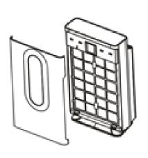
Load the composite filter into the front of the unit and replace the cover.
